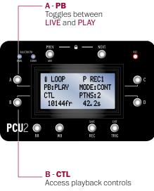
Once in Playback Mode, the first and last frames of the current clip are displayed on the top line. Marked frames appear on the bottom line.
