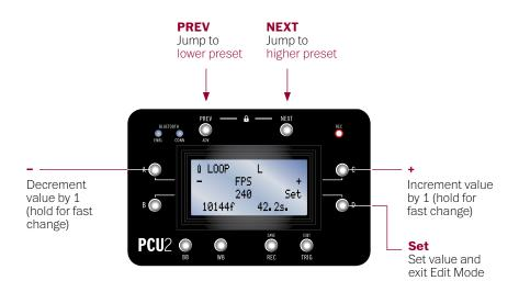
When the parameter is at the desired value, press D, and the PCU will exit Edit Mode.
