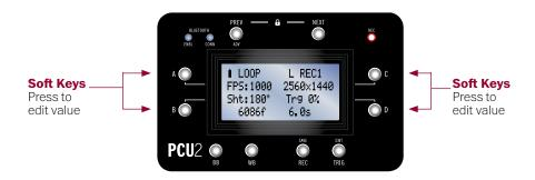
The soft key for a parameter with a wide range of values, such as frame rate, will enter Edit Mode on a new screen (see page 11). The soft key for a parameter with very few potential values will toggle through the options.
