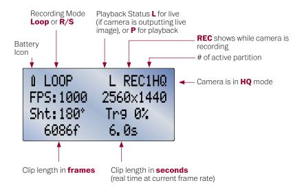
The maximum length of the current shot in frames and real time are displayed on the bottom of the screen.
