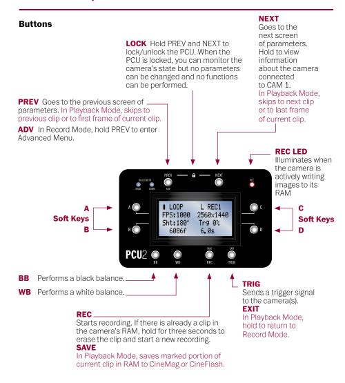
In Record Mode, the PCU2 will show up to four parameters on the screen at once. The parameters can be accessed for editing by pressing the corresponding soft keys to the left and right of the screen.
