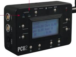
To enable Bluetooth, go to the 'Bluetooth' page of the Advanced menu. The blue LED labeled **ENBL** will illuminate to indicate that Bluetooth is turned on.
