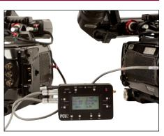
Note: For guaranteed matching in and out points, we recommend using a trigger hard-wired to the trigger ports of each camera. For proper sync, FSYNC must be connected between the two cameras, and a connection should be made between Timecode Out of one camera and Timecode In on the other.
